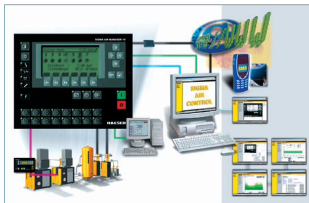
Figure 5. The Sigma Air Manager is a powerful integrated master controller and web server providing everything for effective compressed air management and control.
